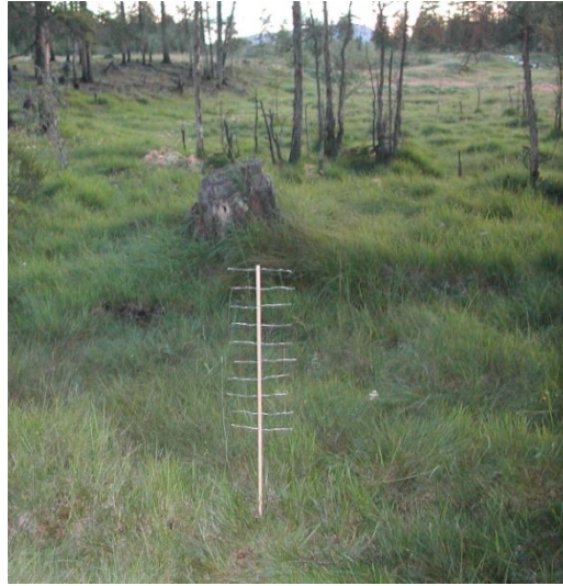
Fig. 2 Simple maximum snow depth gauge
