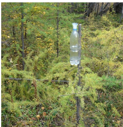
Fig. 1 Simple total rainfall gauge
